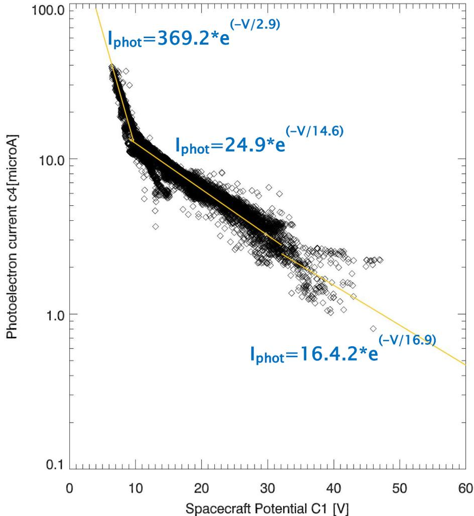
$$\begin{aligned} V < 9 & I_{\text{phot}} = 369.2 * e^{(-V/2.9)} \quad [\mu\text{A}] \\ 9 < V < 32 & I_{\text{phot}} = 24.9 * e^{(-V/14.6)} \quad [\mu\text{A}] \\ V > 32 & I_{\text{phot}} = 16.4 * e^{(-V/16.9)} \quad [\mu\text{A}] \end{aligned}$$
